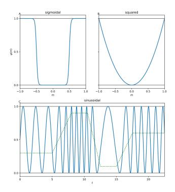
Figure 1: Three functions which depend on motor activity are used to generate sensory interference. Interference determined by the right motor is added to the right sensor's input stream, and likewise for the left sensor and motor. Figures A and B plot pure functions of motor activity, while Figure C plots a function of time whose frequency is determined by the motor activity. The solid blue line shows the interference, while the dotted green line shows the motor activity.
