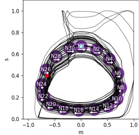
Figure 1: Node positions and sensorimotor trajectory of the robot in Exp. 2. Arrows indicate the  $N_{VA}$  values for each node at end of training. The blue star shows the sensorimotor state at the end of the training phase, and the red circle shows the sensorimotor state at the end of the trial.
